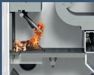
Due to the residual glow zone, re-ignition is quick and efficient. Embers retained during grate cleaning allow for quick ignition.
