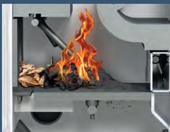
When closed, the tilting grate forms the ideal environment for a bed of embers and thus for optimal combustion.
